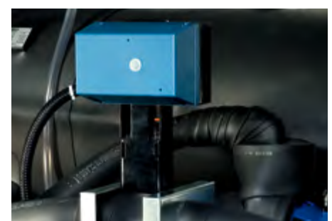
Servo-controlled three-way hydraulic valve.
